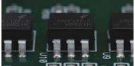
Figure 6. Complete hole-fill of 0.093 inch thick board with ¾ inch thickness solder impingement.
